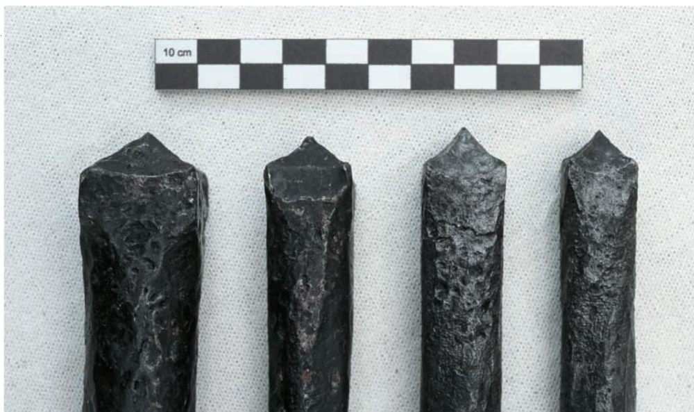
Évolution of fleuret used in mines of Thillot from 1617 AD
