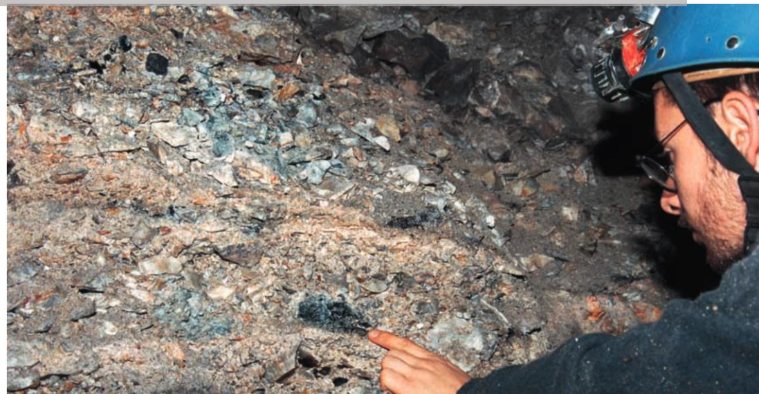
Waste with charcoal issued from fire setting Saint-Roch, L'Argentière-la-Bessée). © Inrap
