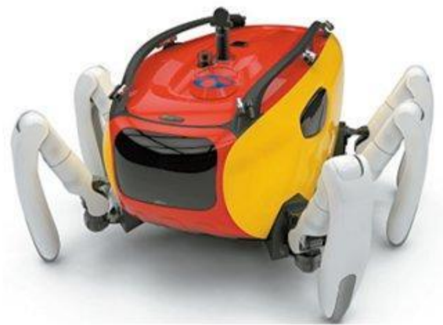
Crabster, robot with sensors for deep water exploration
